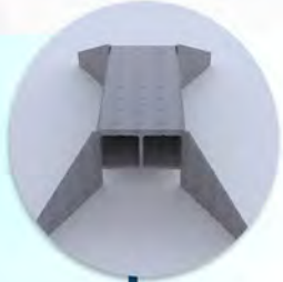
DOUBLE BARREL CULVERT
